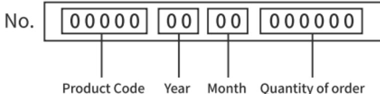
The date of manufacture of the product is encoded in the serial number printed on the body of the tool. The first 2 digits indicate the year of issue, the next 2 digits indicate the month.
